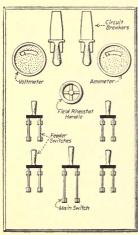
Fig. 204.—Front view of switchboard panel for a single compoundwound direct-current generator.
